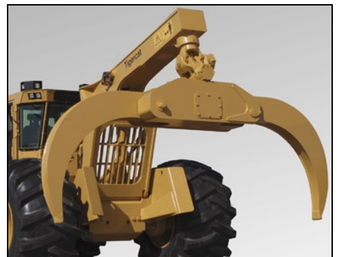
High capacity dual cylinder grapple and grapples and high visibility arch
