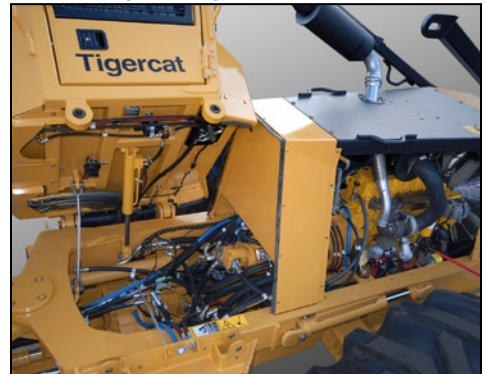
Tilting cab to access pumps and driveline
