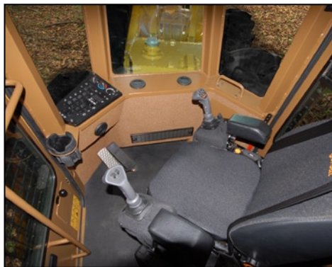
Turnaround™ provides full rear facing drive controls
