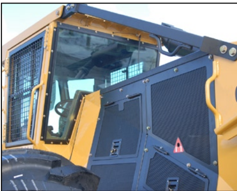
Clear sight line to the sides of the engine compartment
