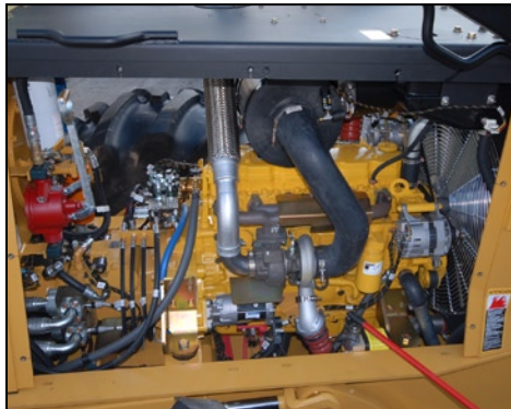
Easy access to both sides of the engine and all service points
