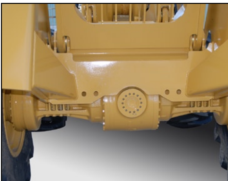
Outboard planetary SFD (severe forest duty) axles are well guarded
