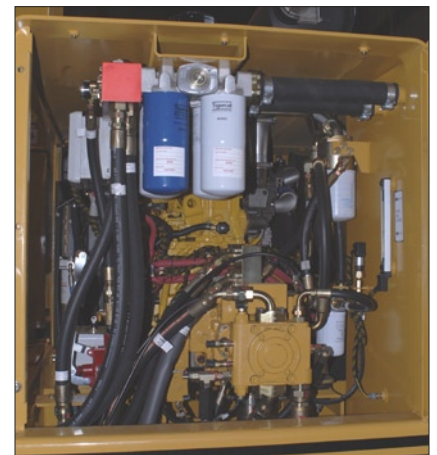
Fuel efficient load sensing hydraulic system
