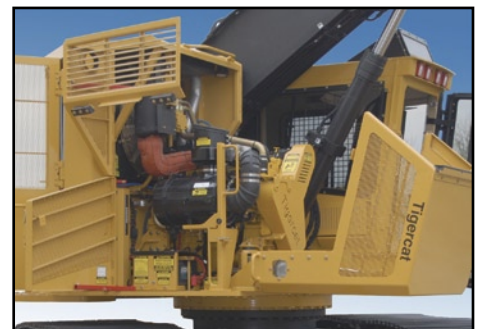
Easy access to the engine through the hydraulically retracting hood enclosure
