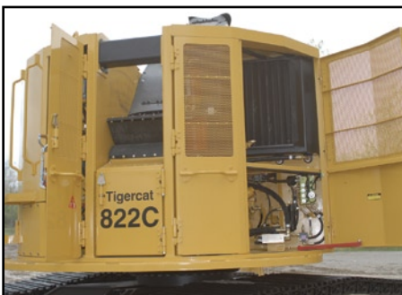
Easy pump access; cooling airflow is drawn from the rear, away from saw debris
