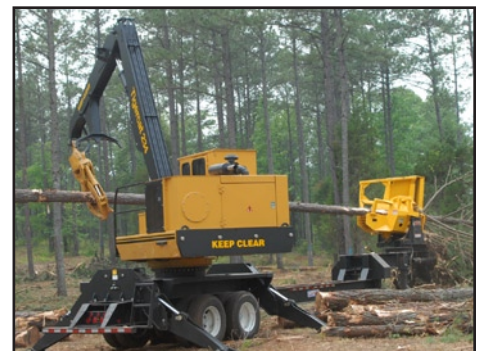
234 and 250B booms resist side stresses and are well suited to heavy duty cycle delimiting applications
