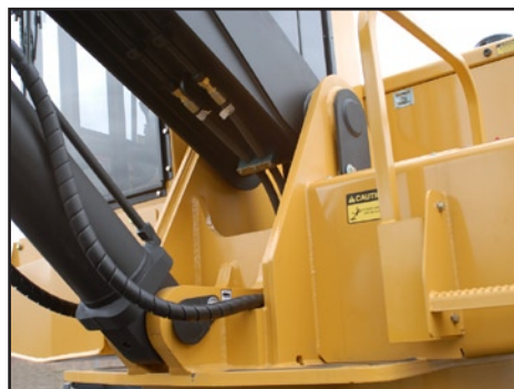
Large pins and thick steel plate at boom pivots
